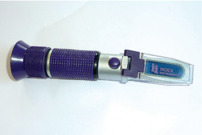
The photo above shows a refractometer. If, for any reason, an engineer does not have one of these, they may not be an appropriate person to carry out the winterisation process.
